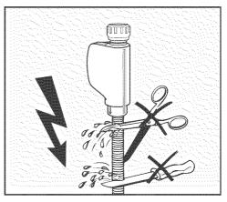
WARNING - Elcetrical Hazard Do not cut the intake hose. If the hose is cut, the dishwasher will not work. There will be a water leak and you could be injured. If the hose is too long, coil it neatly and place it behind the machine.
